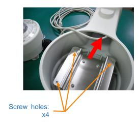
3. Fix the camera to Camera Mount Base with 4 screws (M4 x10).
