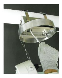
2. Holding the camera, fix it to Pole Mount Adapter in Sunshade with Mounting Screws (M4x10, x4).
