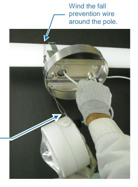
Holding the camera, put the LAN cable from the camera into a through hole of Sunshade Unit.
