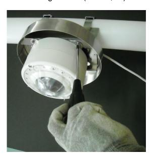
3. After temporally fixing the camera to Camera Mount Base with three screws, cut out the fall prevention wire and then fix all four screws.
