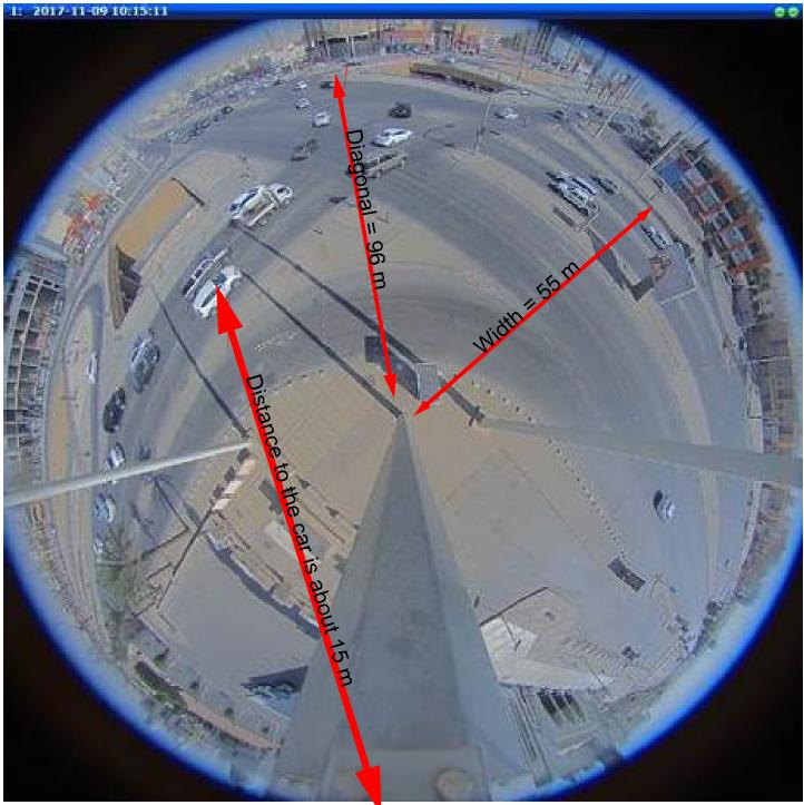
Installed on a pole of 12 m high facing downward.
