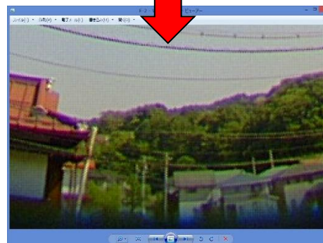
Even with FRIP lens, the image at the fringe area is not sufficiently clear.
